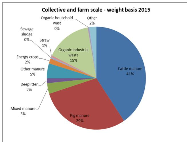
**Figure 3.** The biomass used in the collective and farm scale based biogasplants (Mikkelsen et al. 2016)
