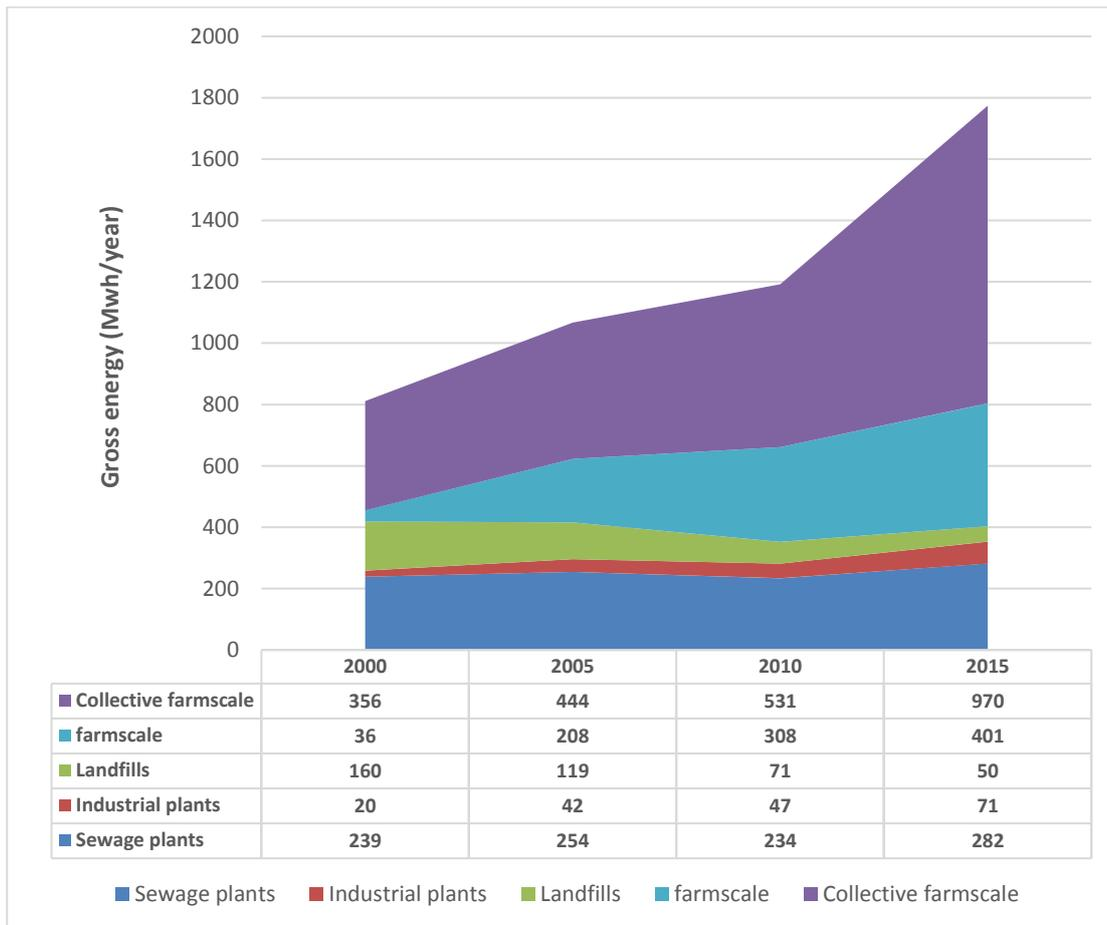
**Figure 2.** Map of gross energy coming from different types of biogas plants in Denmark. The energy is in gross energy without subtracting own consumption at the plants. The farmscale and collective plants co-digest manure with waste.
