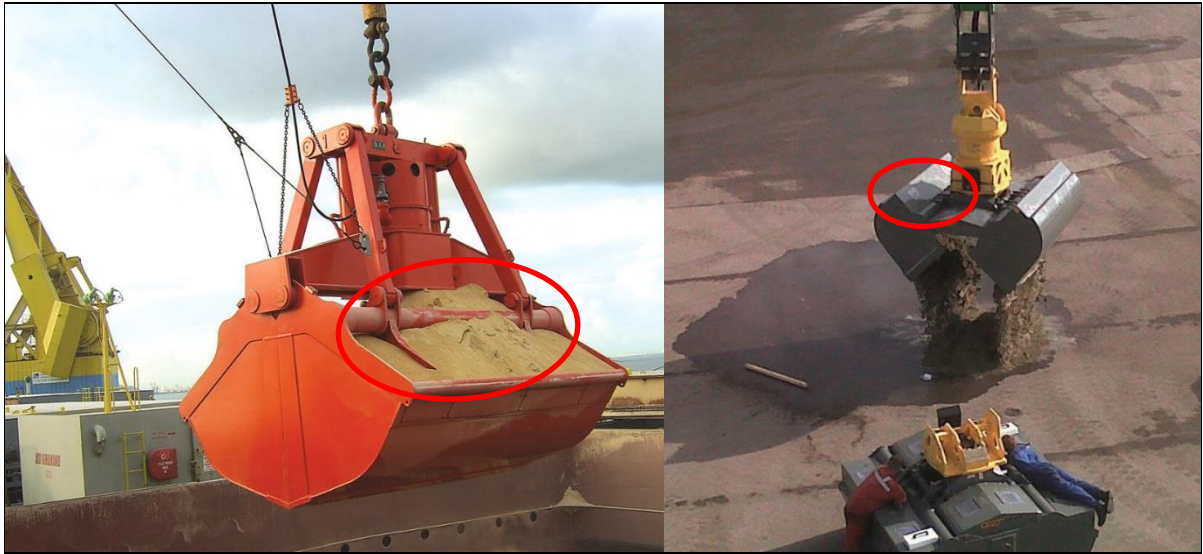
Figure 45: Example of a conventional open-top grab (left) and a closed grab (right)
