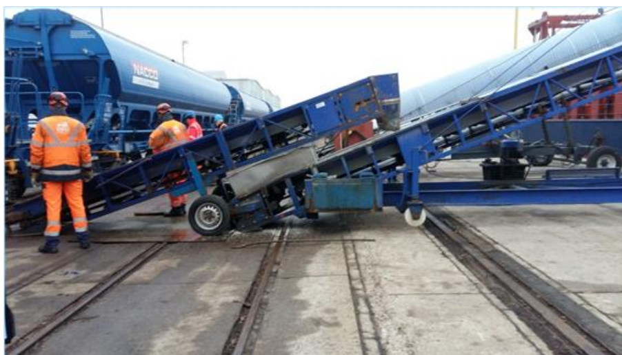
Figure 24: Conveyor belt system between a wagon and a fertiliser loading ship [Ramboll, GER]
