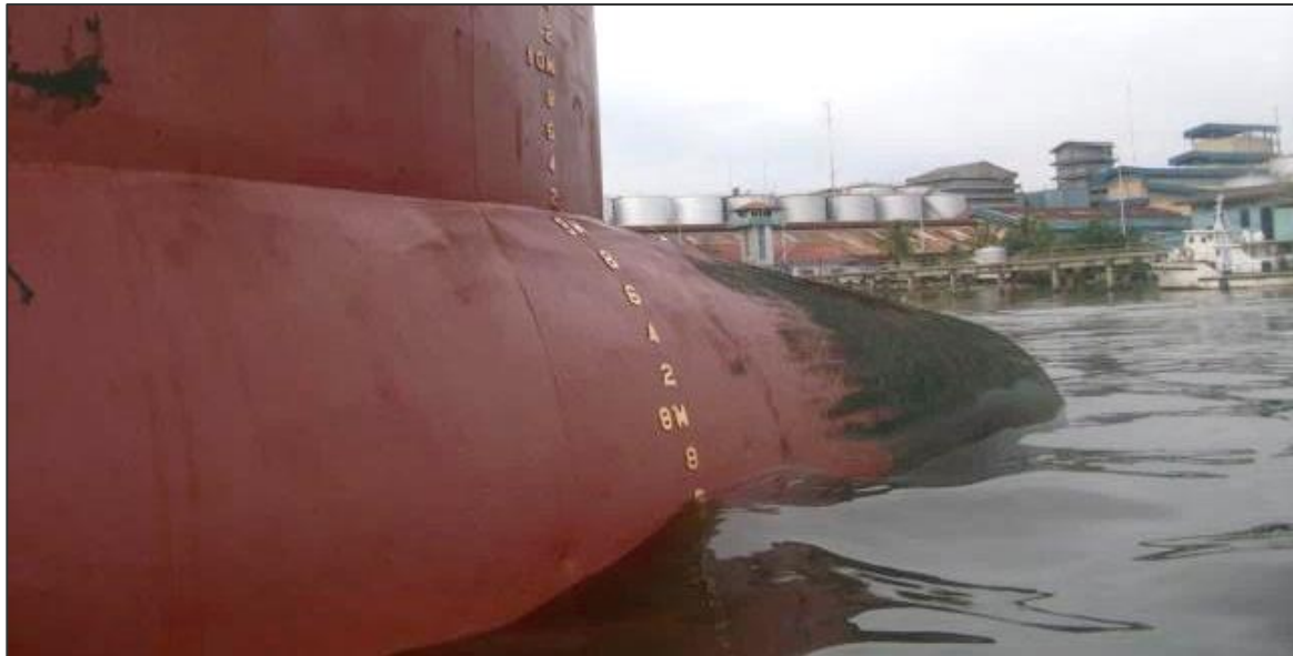
Figure 1: Effect of sea state makes reading draught marks difficult ( https://i2.wp.com/sevensurveyor.com/wp-content/uploads/2011/01/Draftmark.jpg )
