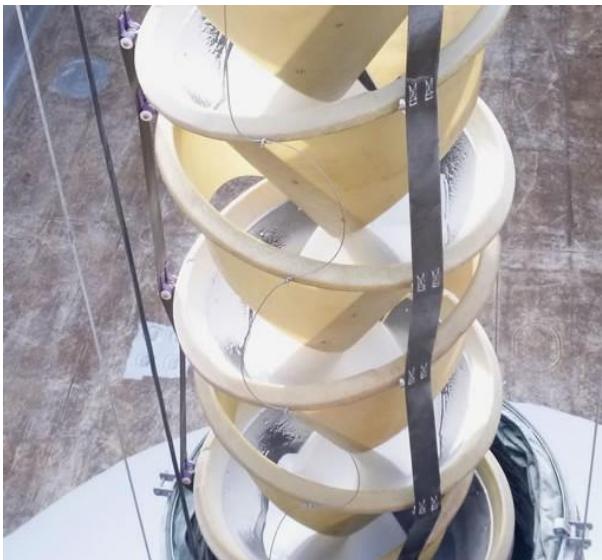
Figure 51: Principle of cascade chutes ( http://clevelandcascades.co.uk )
