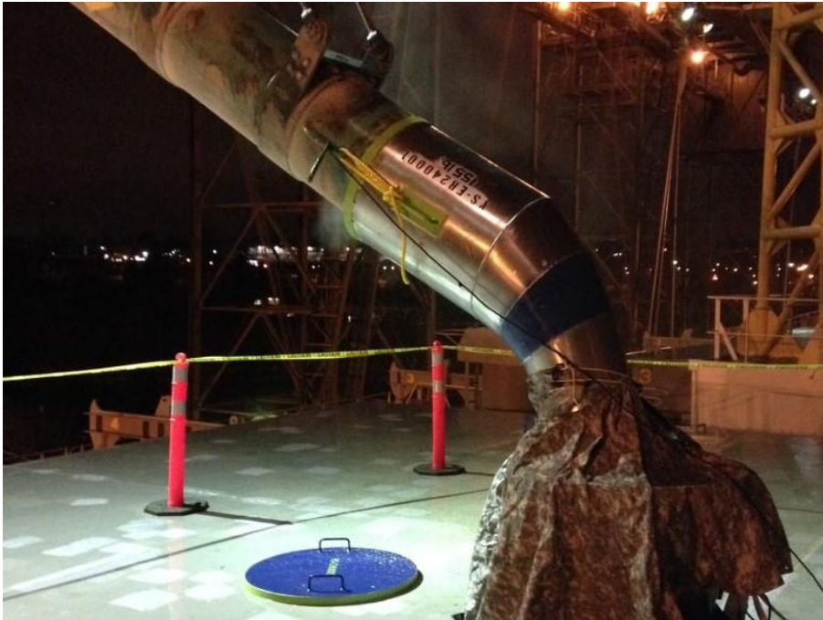
Figure 53: Example of using feeder holes on the hatch cover ( https://www.colleywest.bc.ca/feeder-hole-loading-2/ )
