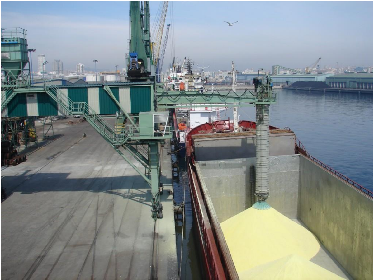
Figure 52: Example of a ship loader with a cascade chute. Note the smooth box-shaped hold. ( http://clevelandcascades.co.uk )
