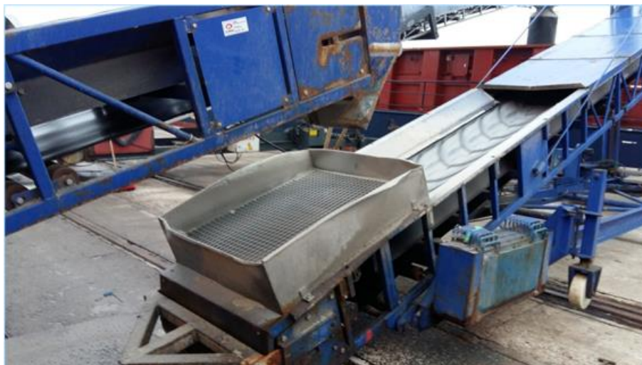
Figure 26: Strainer between parts of a two-belt system [Ramboll, GER]
