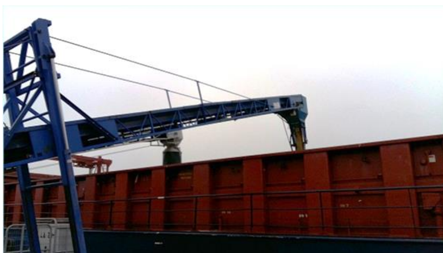
Figure 27: End of the second belt forwarding fertiliser onto the ship [Ramboll, GER]
