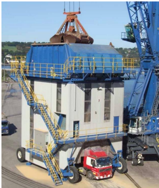
Figure 46: Example of a hopper with a special dust management system ( http://www.docksolid.com/ )
