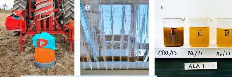
**LABORATORY ANALYSES:** 1 Drilling of soil monoliths 2 Simulation of rainfall 3 Samples of runoff water. Photos: Natural Resources Institute, photo archive.
