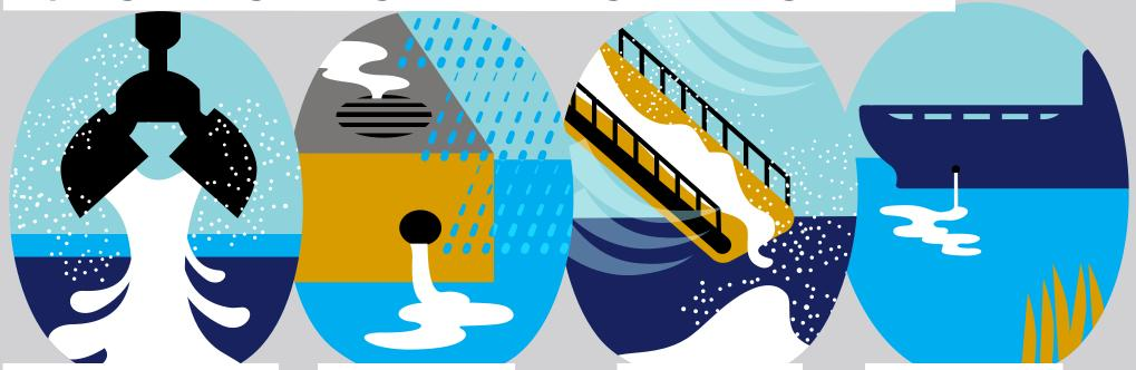
Fertilizer will scatter in the air and fall off from a clamshell grab if the grab is in a bad condition, packed too tightly or opened too high up.
