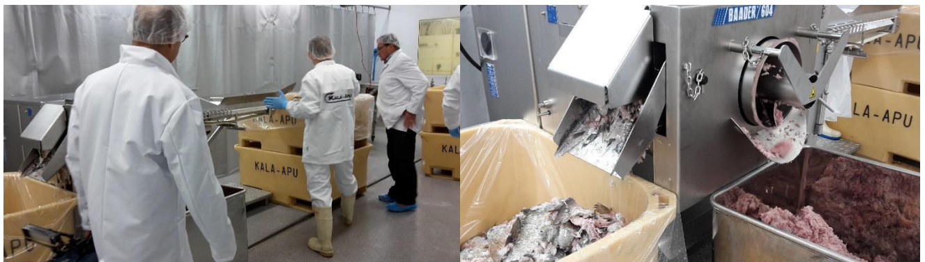
Figure 4. Kala-Apu Oy's mincing machine separates the skin and bones from the fish. Images: John Nurminen Foundation
