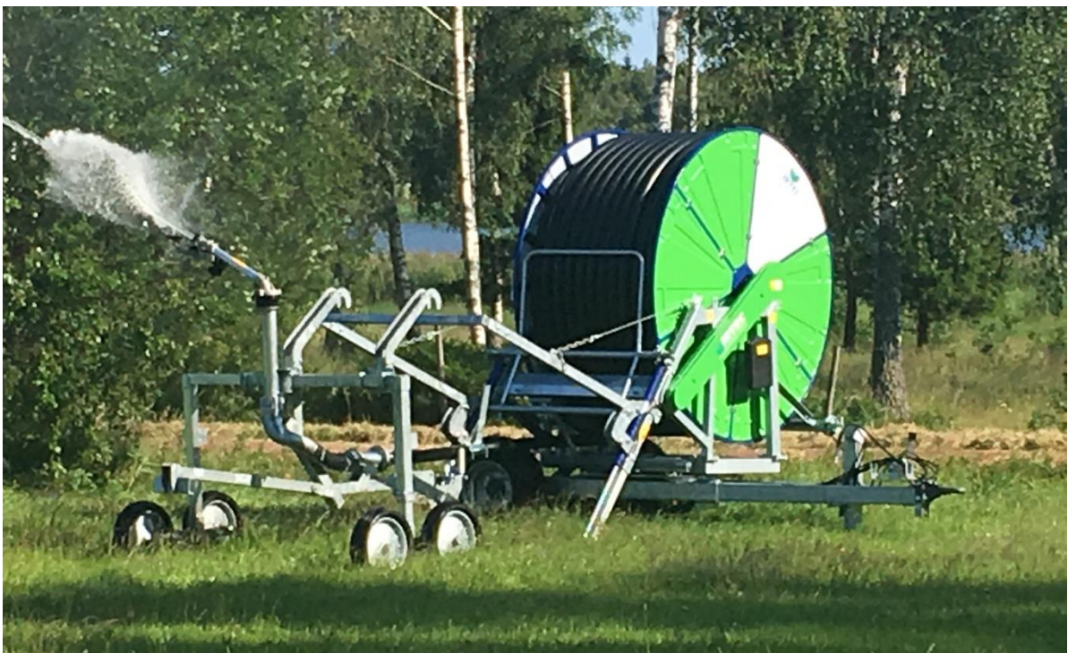
An irrigation water cannon. Photo: Annica Brink
