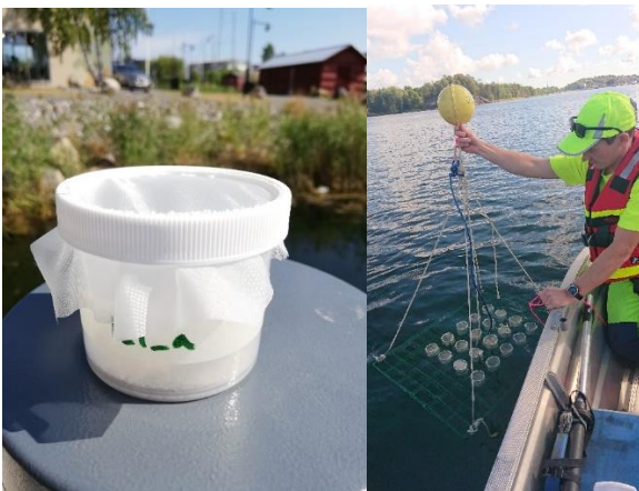
Figure 5.3 Left: Picture of the experimental bottle with 90 µm netted mesh under drilled out lid. The bottom of the bottle is covered by marl sorbent. Right: Deployment of a set of experimental bottles in Farstaviken Bay
