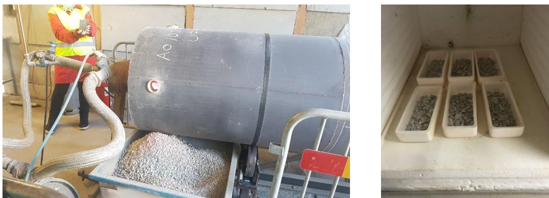
Figure 7.1 Left: Rotating furnace used for production of marl sorbent for the field trials. Right: Muffle furnace used for production of marl sorbent for the laboratory studies.
